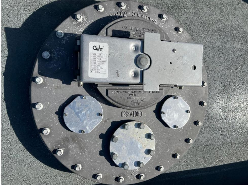
The European standard manhole is installed on the top of the tank , with built-in breathing and emergency exhaust function, the built-in breathing valve keeps the internal pressure of the tank stable during the fuel transportation process, and achieves balance with the external pressure.Prevent overflow design to seal the tank in case of accident.
