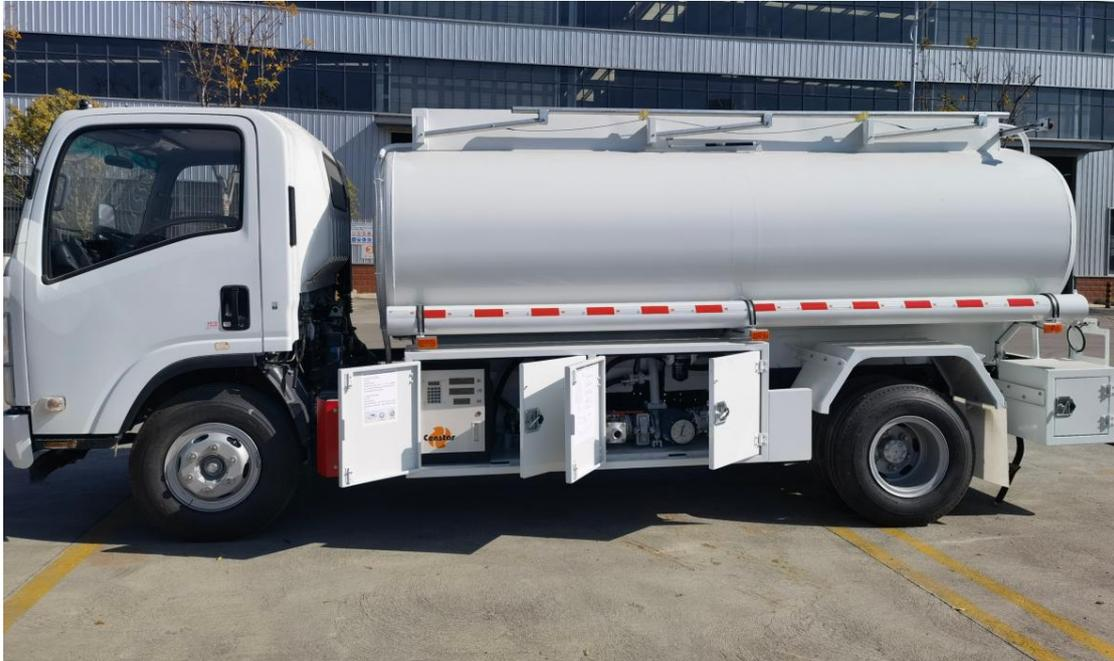
The fuel tank is made of high-quality steel plate with square cylinder structure. The whole tank is single compartment. There are through holes at the lower end of the middle baffle plate. The middle of each compartment is welded with strengthened wave proof baffle plate to reduce the impact of fuel in the tank and improve the rigidity of the tank body when driving.
